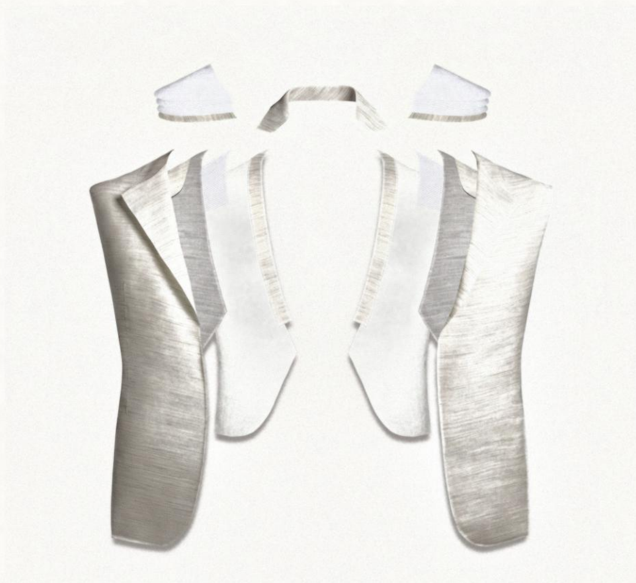
OUTER CLOTH · CANVAS OR FUSIBLE · CHEST PIECE · SHOULDER PAD · SLEEVE HEAD · LINING
